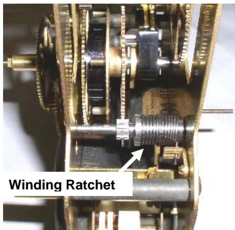
The winding ratchet is a spring-friction affair. It offers substantial resistance to movement. However it also could not be adjusted for less resistance without negatively affecting the winding efficiency or function.
