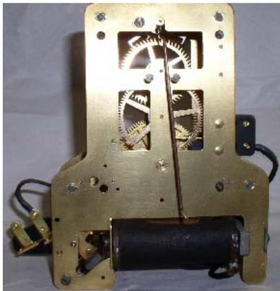
The plates are marked "1418-V." The coils on the clock are marked 10V. The owner insisted that the clock was marked as 10 volts. However it must be noted that we could not, no matter what we tried, get this unit to wind correctly, let alone efficiently on 10 volts. It would simply quiver, but would not wind strongly. No contact adjustment was of help in curing the problem. Coil resistance was 80 ohms. Our experience with Model 45 movements is that the 10 volt versions were 30 ohms.
