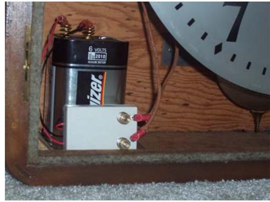
**Above left: Model 1000R** converter. This configuration fits into every self-winding clock we could find. At right: The Model 1000 powering a Self-winding clock from a 6V lantern battery. This arrangement will yield close to 2 years of life from the battery.
