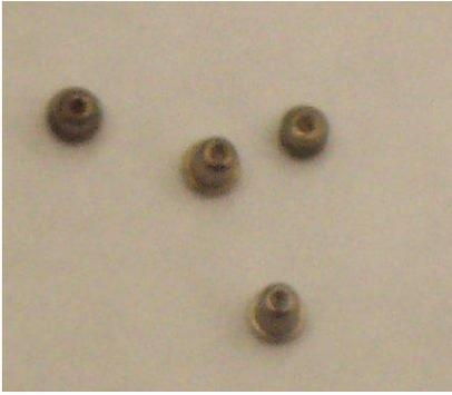
it's almost certain these cups will need to be refitted. And, most certainly the balance staffs will need to be turned on a lathe and resharpened. Neglecting this repair will result in erratic timekeeping or even a clock that will not run for more than a few hours.
