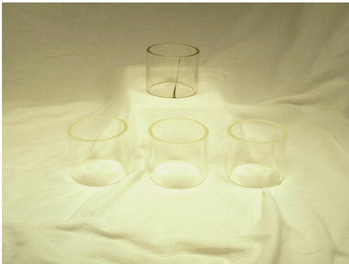
**Glass Sleeves.** Shown in the foreground are three cut sections of glass sleeve to be used as Spider cases. The diameter of these sleeves is about 1mm smaller than the original sleeve, which is not noticeable once installed in the clock. This standard Simax product, cut to size, makes a nice replacement for broken or missing Spider glass cases. An original broken Spider case is shown in the back.
