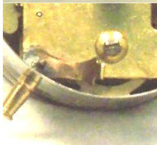
The "click" is a pair of flimsy brass tabs protruding from the pillars of the movement as shown in the inset. We have only seen one original undamaged click out of the many clocks we've examined. Usually they have been soldered onto the pillars (as is shown here) because the original staking had come loose or the click had broken off at the base. Most of the
