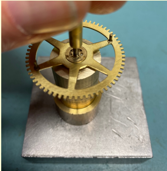
1" brass cutoff Drilled to accommodate Trundle cage
